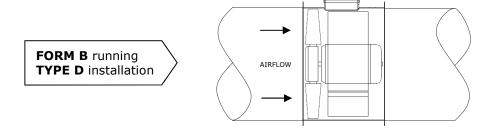
Form A running shall have the airflow in the opposite direction of Form B.
