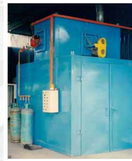
Paint Drying Oven
