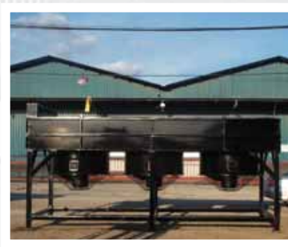
Horizontal remote radiator that comes with motor and fan and the air flows vertically upwards
