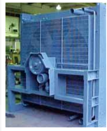
Set mounted radiator where fan is mounted on radiator and driven via pulley and belts
