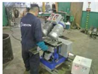
SELF PROPELLED PLATE BEVELLING
