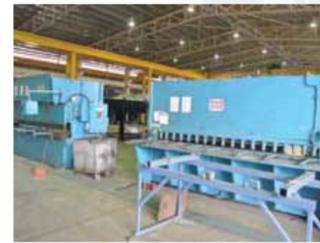
NC BENDING & SHEARING MACHINE
