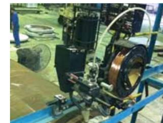
SUBMERGED ARC WELDING MACHINE
