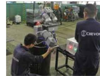
SELF PROPELLED PLATE EDGE MILLING
