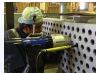
PORTABLE ELECTRICAL TUBE TO TUBESHEET/
